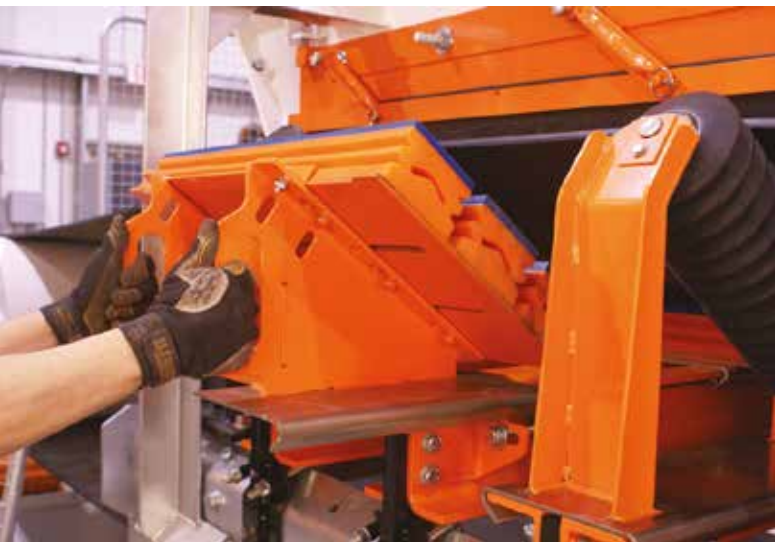
Designed for ease of service, modular components allow faster, safer change-outs by one person
