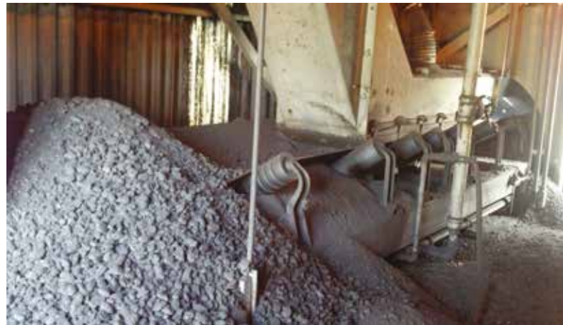
If the spillage rate is just 4 grams per minute, the accumulation will be more than two tons per year
